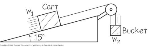
When released, the cart accelerates up the ramp and the bucket accelerates downward. How does the cable tension *T* compare to  $w_2$ ?
