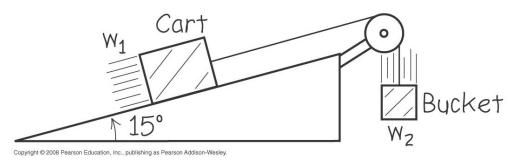
When released, the cart accelerates up the ramp.
